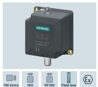
SIMATIC RF350R is a universal reader for operation with external antennas. Due to the different, pluggable antenna designs (flat antenna, round antennas), there are many possible applications in the area of industrial production, especially in assembly lines. This reader has an RS422 interface with transmission procedure 3964R for connection to the RFID communication modules ASM 456, ASM 475, SIMATIC RF160C, RF170C, RF180C and RF182C.
