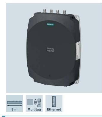
SIMATIC RF670R is a high-performance RFID reader with four antenna connections which can be configured as required for individual read stations, detecting at conveyor systems, or as gates. The high transmit power of up to 2 W ERP / 4 W EIRP (dependent on antenna and cable) permits large ranges of up to 10 m in gate applications. The high degree of protection of the overall system is a guarantee for problem-free use, even under the most difficult environmental conditions.
