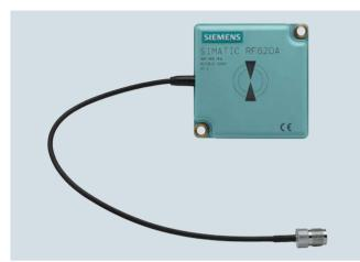
The SIMATIC RF620A antenna is characterized by an especially compact enclosure. It is particularly suitable for use in production, e.g. on assembly lines or track-guided conveyor systems. The effects of reflections and overshooting can be reliably reduced thanks to the linear polarization and high degree of signal attenuation.
