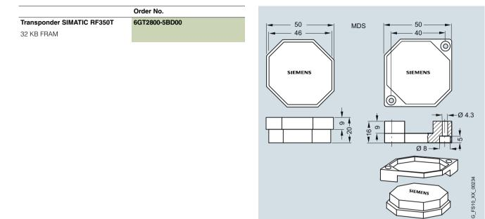
Left: Transponder SIMATIC RF350T. Top right: Mounting frame. Lower right: Installation diagram. The transponder can be mounted with the mounting frame as shown.
