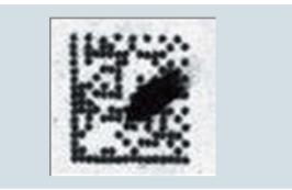
Damaged surface of the marking or part
