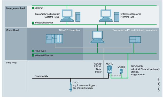
Integration of SIMATIC MV420/MV440 with connection via RS232
