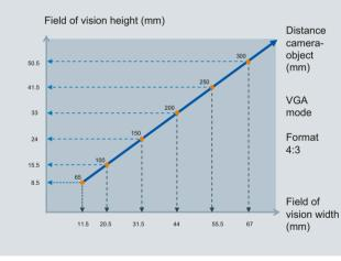
SIMATIC MV420 field of view dimensions for the 16 mm lens Further information can be found in the supplied manual.
