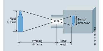
The required image field size (height and width of the image), the size of the sensor chip and the focal length of the lens determine the operating distance:
