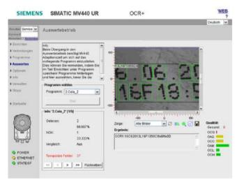
With the "Text-Genius" and "Text-Genius Plus" licenses, SIMATIC MV440 can be used for text recognition (in addition to reading 1D bar codes and 2D matrix codes). Text recognition is also referred to as OCR (Optical Character Recognition). Simultaneous reading and comparing of plain text and reading of machine-readable codes in the same image field is thus possible.
