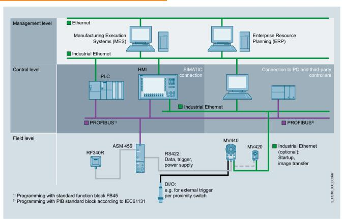
Integration of SIMATIC MV420/MV440 by means of the ASM 456 communication module
