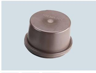
Heat-resistant, rugged transponder for use in paint shops (automobile industry, primer/top coat) or applications with similar temperature requirements, memory capacity 32 KB RAM, temperature range -25 °C to +85 °C, up to +220 °C cyclically, IP68 degree of protection, enclosure dimensions (mm) Ø 114 x 83.
