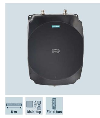
The UHF RFID reader SIMATIC RF630R has been specially designed for the requirements in production. The reader can be used with one or two external antennas (SIMATIC RF620A/640A/642A/660A). The device is integrated into automation systems via the RS422 system interface. Connection to PROFIBUS, PROFINET, and Industrial Ethernet or directly to SIMATIC S7-300 is supported (via communication modules SIMATIC RF170C/180C/182C or ASM 456/475).
