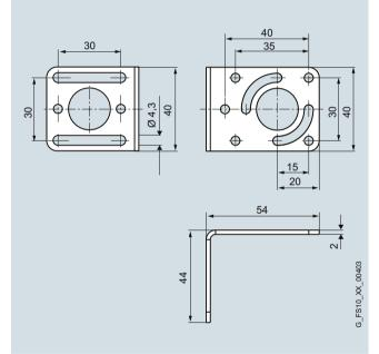
Mounting bracket for code reading system SIMATIC MV420
