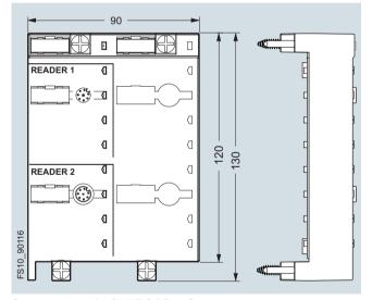
Connector block for SIMATIC RF170C
