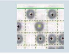
Incorrect or non-uniform cell position in the marking
