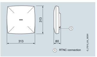
SIMATIC RF660A antenna, position of connection
