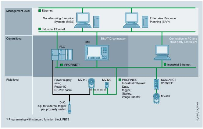
Integration of SIMATIC MV420/MV440 with a direct connection to PROFINET or Ethernet
