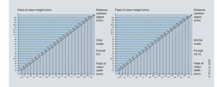
SIMATIC MV420 field of view dimensions for the 6 mm lens
