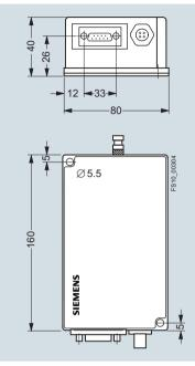
SLG D11 / SLG D11S reader basic unit
