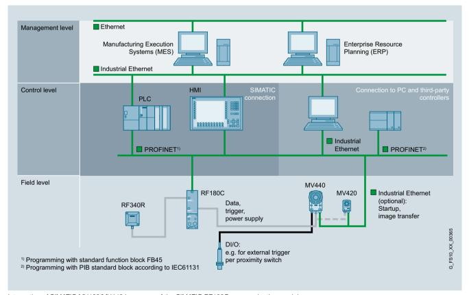
Integration of SIMATIC MV420/MV440 by means of the SIMATIC RF180C communication module
