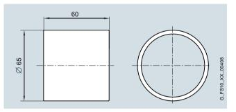
Protective barrel for lens D65
