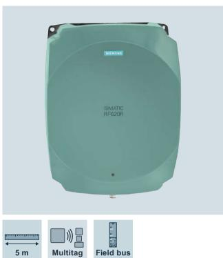
The UHF RFID reader SIMATIC RF620R has been specially designed for the requirements in production. The reader has an integral antenna and thus reduces the installation requirements compared to devices with an external antenna connection. The device is integrated into automation systems via the RS422 system interface. Connection to PROFIBUS, PROFINET, and Industrial Ethernet or directly to SIMATIC S7-300 is supported (via communication modules SIMATIC RF170C/180C/182C or ASM 456/475).
